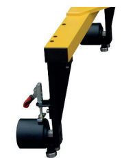
Elevated trolley for slab track construction using iron horses
